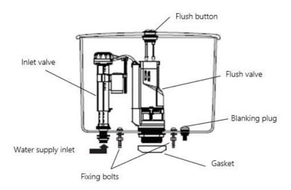
5. Position the cistern onto the pan by centring the gasket on the pan inlet and then secure the cistern in position using the fixing bolts.
