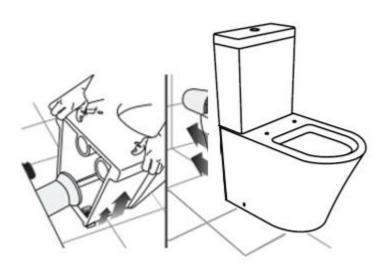
8. Ensure the pan is level and then secure it to the fixing brackets using the pan fixing screws and washers provided. Fix on the cover caps.
