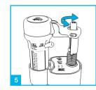
The water level can be adjusted by turning the adjustment screw (clockwise for more water, anticlockwise for less water).
