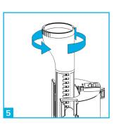
To adjust the overflow tube height, turn tube anticlockwise and adjust up and down to the correct position. Turn clockwise to lock into place.
