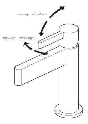
Moving the mixer lever upwards/downwards will increase/decrease the flow of water. Moving the mixer lever from right to left will increase the water temperature.
