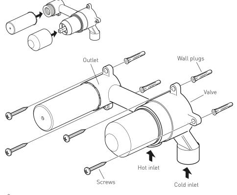
**Warning!** Please check for any hidden cables and pipes before drilling holes in the wall.
