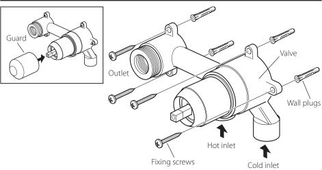
Before installing your new mixer, flush through the pipe work to ensure removal of debris, turn off the water supply.
