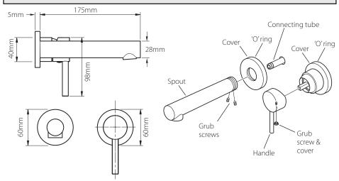
Slide the cover over the valve, push onto the wall until it makes contact.
