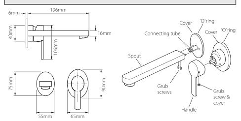
Slide the cover over the valve, push onto the wall until it makes contact.
