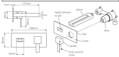
Using sufficient ptfe tape to hold the spout securely and prevent leaks, screw the spout into the valve body and adjust the spout to the correct position for when the cover is slid on.
