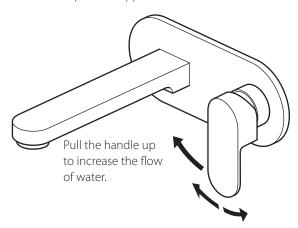
Turn the handle clockwise to increase the temperature and anti-clockwise to decrease the temperature.
