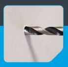
Drill a 10mm hole in the substrate.
