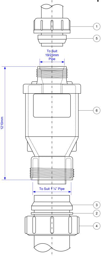
Connect 19/23mm Pipe into Part 6 Using Nut, 1, and Seal 5 in order and position shown above.
