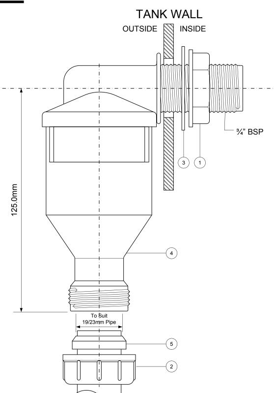
Install Tun Dish onto Tank by assembling Parts 1, 3 & 4 in positions indicated.
